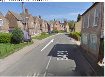
Currently there are speed cushions on the section of the B489 High Street to the east of Brookmead School, which whilst only provide a modest speed reduction effect, act as a physical reminder to drivers to slow down. The removal of these is likely to lead to an increase in vehicle speeds, particularly of vehicles travelling on the downhill westbound approach to the school, which may result in speed related collisions.
